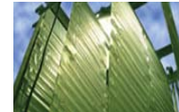
Fig. 6: Right: Vertigo, developed by Global Green Solutions. Consists of racks of plastic tubing.
