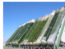
Fig. 7: Below: GreenFuel technologies' bioreactor in AZ, which uses power plant emissions.
